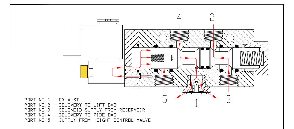
WHEN THE SOLENDID IS ACTIVATED, AIR PRESSURE FROM PORT ND. 3 (RESERVOIR)BUILDS, MOVING THE SPOOL OVER CLOSING PORT ND. 5. THIS ALLOWS PORT ND. 4 (LIFT AXLE RIDE BAGS) TO EXHHAUST WHILE SIMULTANEOUSLY ALLOWING THE LIFT AXLE BAG TO INFLATE (PORT ND. 2) RAISING THE LIFT AXLE.
