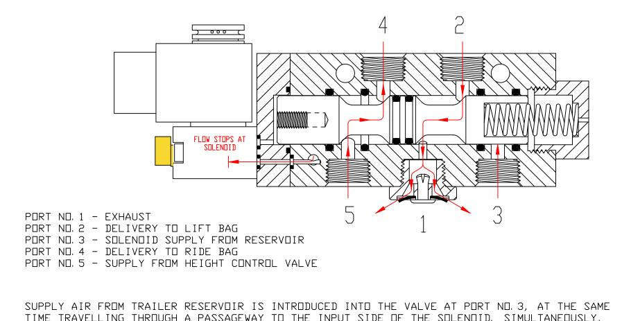
SUPPLY AIR FROM TRAILER RESERVOIR IS INTRODUCED INTO THE VALVE AT PORT NO.3, AT THE SAME TIME TRAVELLING THROUGH A PASSAGEWAY TO THE INPUT SIDE OF THE SOLENOID. SIMULTANEOUSLY, AIR FROM FROM THE HEIGHT CONTROL VALVE IS INTRODUCED AT PORT NO.5 PASSING THROUGH THE VALVE AND EXITING AT PORT NO.4. THIS AIR FILLS THE RIDE BAGS WHICH LOWERS THE LIFT AXLE. WHILE THE RIDE BAGS ARE FILLING, THE LIFT BAG IS EXHAUSTING THROUGH PORT NO. 1
