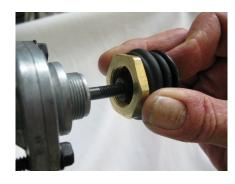
Tighten nut to securely. Make sure boot overlaps knob by at least 1/4".
