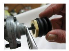
Hold preassembled nut, boot and knob assembly in other hand.
