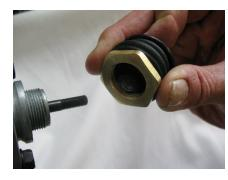
Thread retainer nut on to valve body threads.
