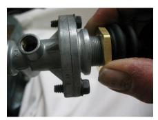
Align assembly and thread knob on to knob shaft.
