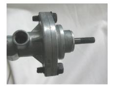
Twist knob eight or more turns on to shaft. Hold shaft with pliers if needed.
